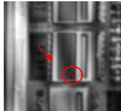
Figure 2: Dice with JTAG failure was detected a significant signal by IR-OBIRCH technique.
