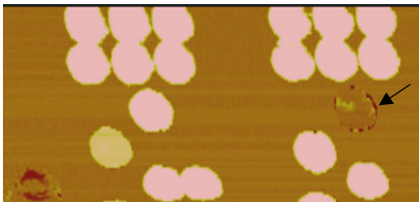
Fig 5 (b) SCM imaging of identical contacts from a bad write driver. The arrow shows the location of the bad contact.
