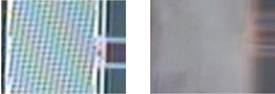
Figure 9a,b: Image a) At zoom= ~50, light- ~8, the optical microscope is re-focused up from the surface. Image b) is about 20microns 'over' the sample. The tips are about 1mm above the surface.
