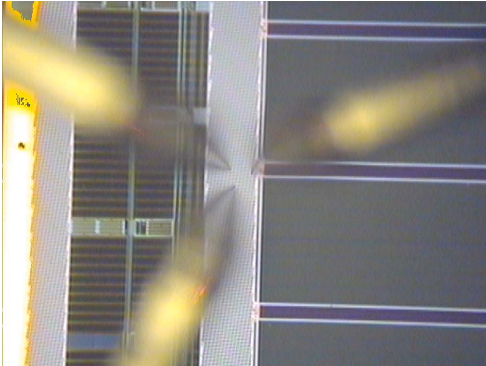
Figure 20: Optical microscope view of the probes in position to image the corner of the array. The corner is a unique feature appearing in each of the scanner images that serves as an alignment mark for registering the relative head positions.
