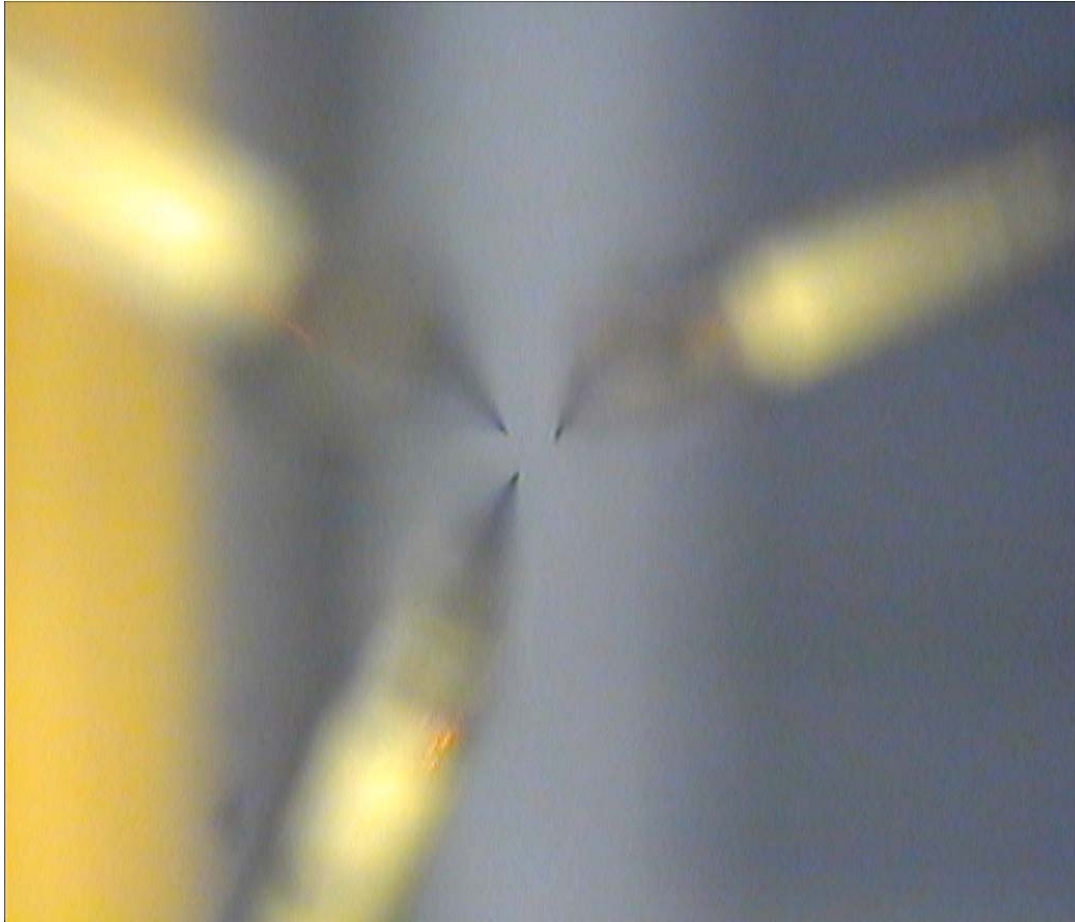
Figure 3: A head is raised to the probe-exchange position before changing probes.
