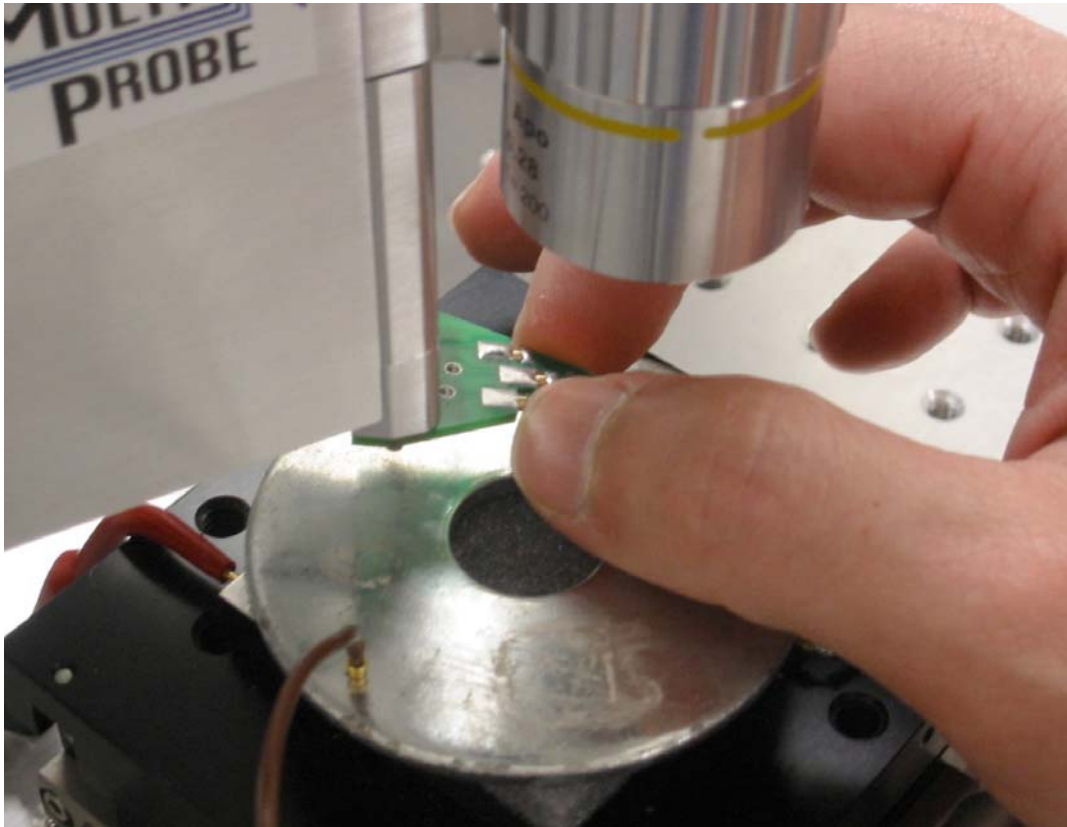
Figure 6: Manually verify tip board is secure.
